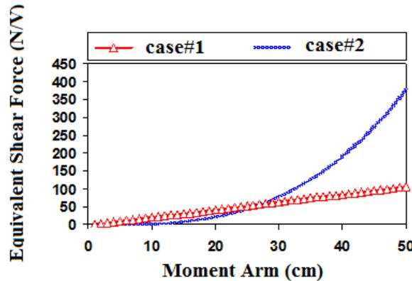
Figure 4. Comparison of control force in two cases with regard to change of moment arm.
