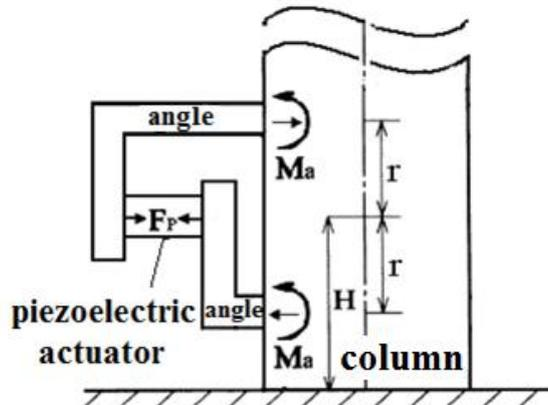
Figure 3. Piezoelectric actuators placement in case#2.
