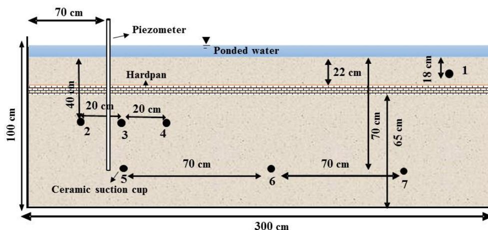
**Fig. 2.** Lysimeter, ceramic suction cup and piezometer.
