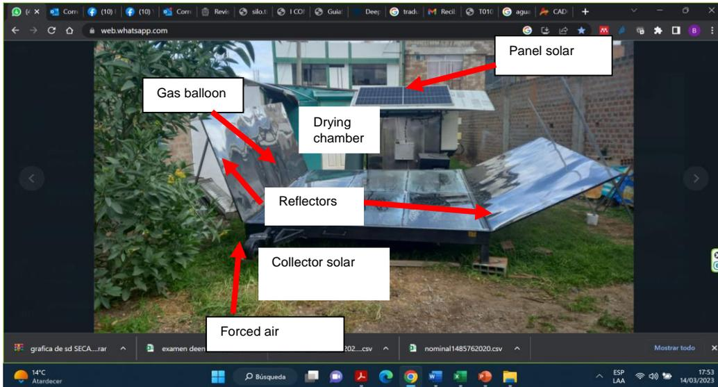
Fig. 2. Dual sun and gas dryer.
