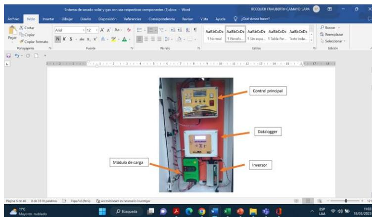
Fig. 3. Control cabin of the solar and gas dryer.
