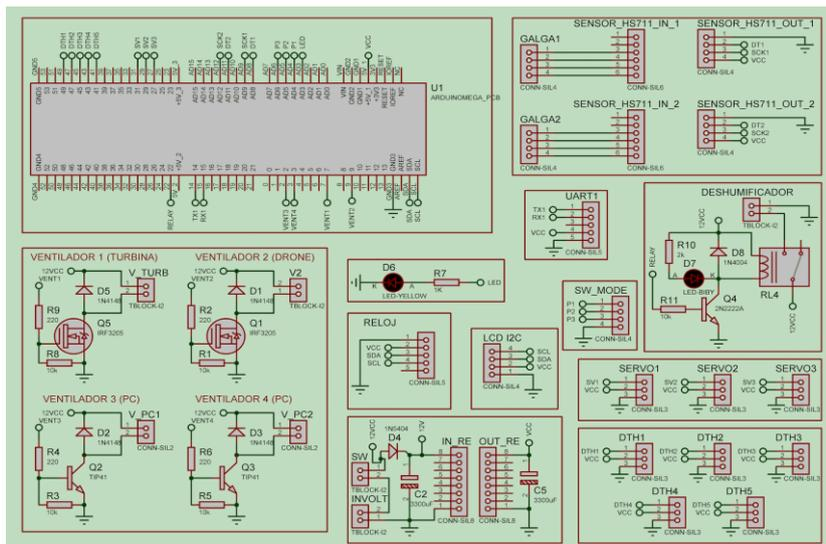
Fig. 4. Main Master Control Board.
