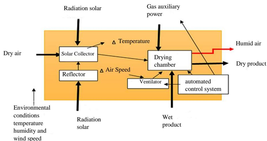
Fig. 1. White box of an indirect solar dryer.
