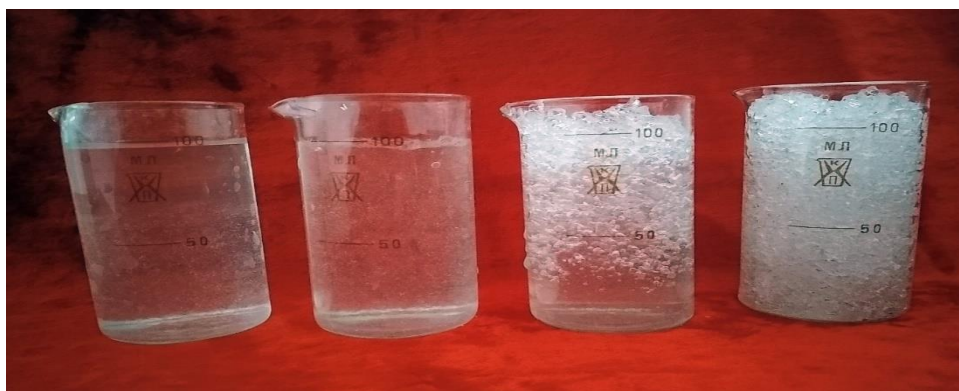
Fig. 2. Gels formed from STOCKOSORB hydrogel mixture in distilled water at pH 5, 7 and 9; 70% in glass 1 from left; 100% in glass 2; 110% in glass 3; 120% volume gels in glass 4.
