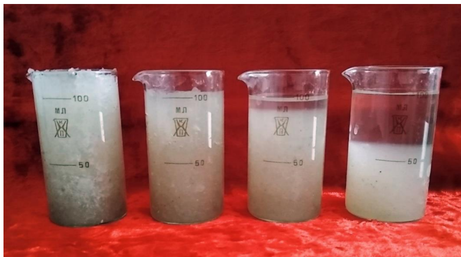
Fig. 3: Gels formed from a Mujiza hydrogel mixture in a distilled water at pH 5, 7 and 9; From right gels of 60% in the 1 st glass, 80% in the 2 nd glass, 100% in the 3 rd glass, and 120% in the 4 th glass.
