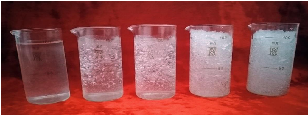
Fig. 1: Gels formed from AQUASORB hydrogel mixture in distilled water medium pH 5, 7 and 9, 80% in glass 1 from left; 90% in glass 2; 100% in glass 3; 110% in glass 4; and view of gels at 120% volume in glass 5.
