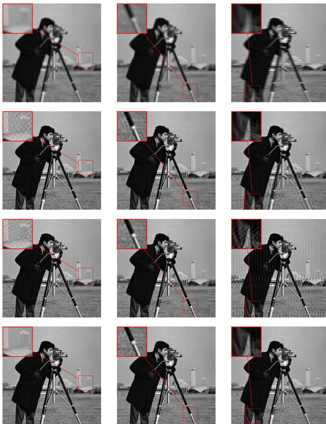
Figure 4: Deconvolution of Cameraman image. From left to right, the first column represents degradation by kernel 1, the second column for the degradation by kernel 2, and by kernel 3 in the third column. From top to bottom, the order of the rows is as follows: blurred images using the three kernels respectively, restored images using blind Richardson-Lucy algorithm [12], restored images using iterative Wiener filter method [3], and finally the restored images using our proposed blind MAP- H^1 model.
