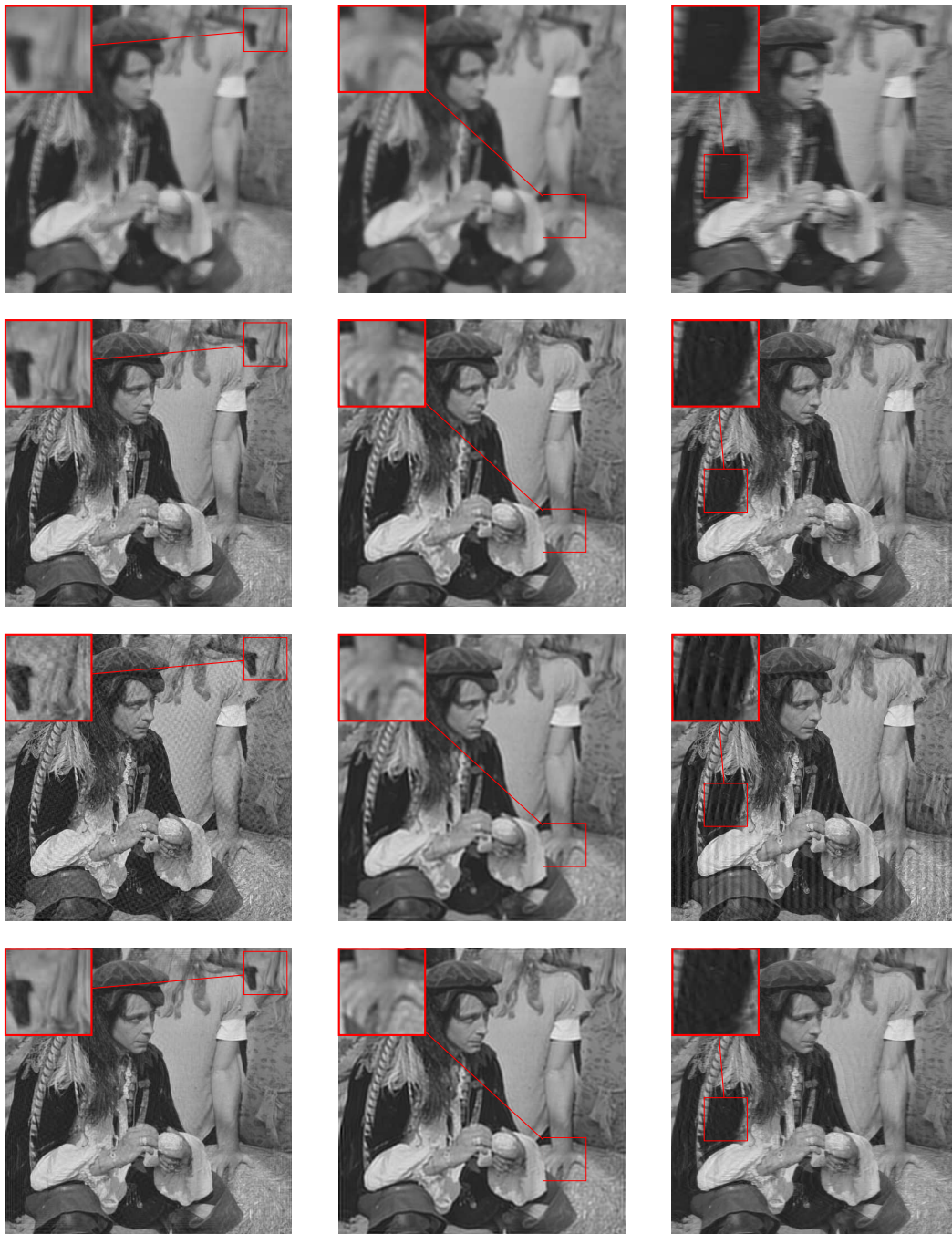
Figure 7: Deconvolution of Pirate image. From left to right, the first column represents degradation by kernel 1, the second column for the degradation by kernel 2, and by kernel 3 in the third column. From top to bottom, the order of the rows is as follows: blurred images using the three kernels respectively, restored images using blind Richardson-Lucy algorithm [12], restored images using iterative Wiener filter method [3], and finally the restored images using our proposed blind MAP- H^1 model.
