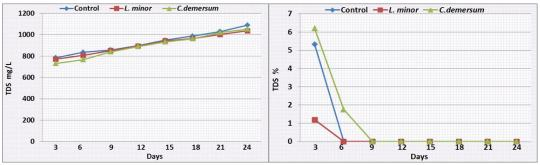
Figs. 4 A-B. Concentrations and rate (%) of bio-removal of TDS (mg L<sup>-1</sup>) during remediation.
