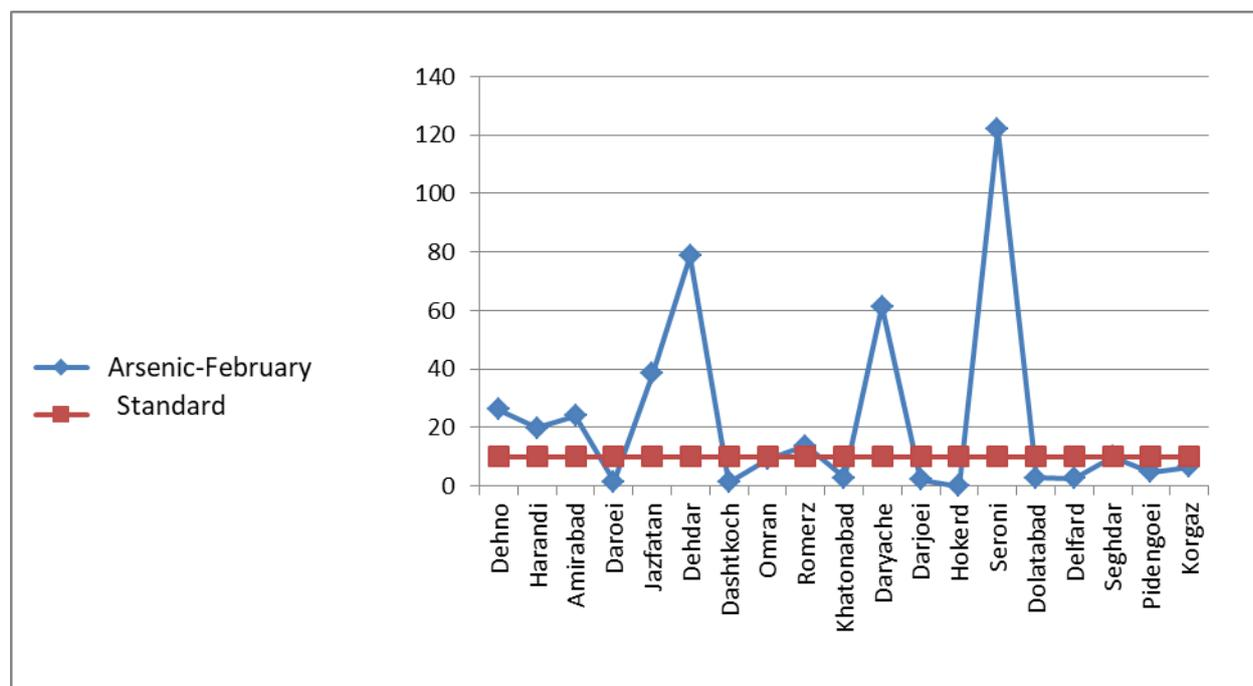
**Fig. 4.** Comparison of arsenic concentrations with standard values in February 2017.
