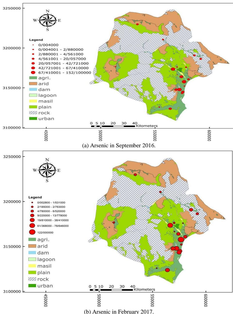
**Fig. 6.** Hot spot analyses exhibiting the relationship between land-use and arsenic concentration (Standard, deviation = 213).
