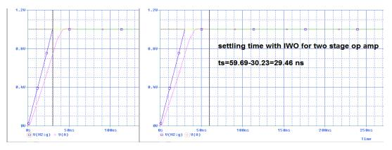
Figure .16. Simulation result of settling time measurement
