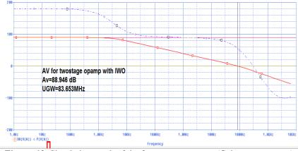
Figure .13. Simulation result of the frequency response (Gain measurement)
