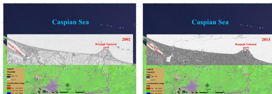
Fig. 7. Shoreline configuration using Laplacian filter from 2002 to 2013.
