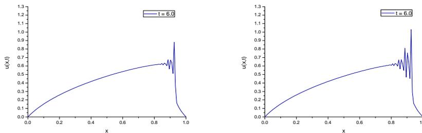
Figure 18: HWCM solution for  $\alpha = 2$ ,  $j = 2$ ,  $\epsilon = 0.0001$  (left) and  $\epsilon = 0.0000001$  (right) with  $\Delta t = 0.001$ .
