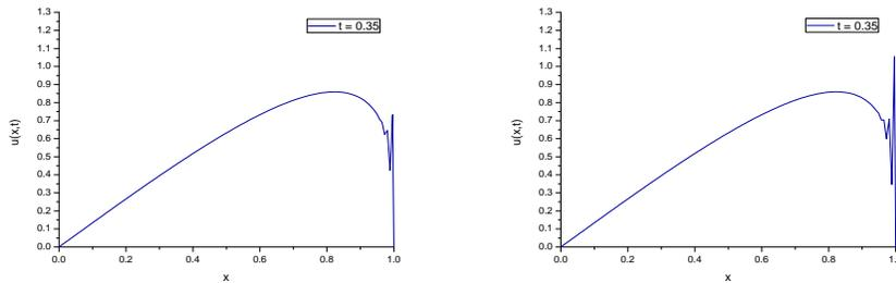
Figure 14: HWCM solution for  $\alpha = 1$ ,  $j = 1$ ,  $\epsilon = 0.0001$  (left) and  $\epsilon = 0.0000001$  (right) with  $\Delta t = 0.001$ .
