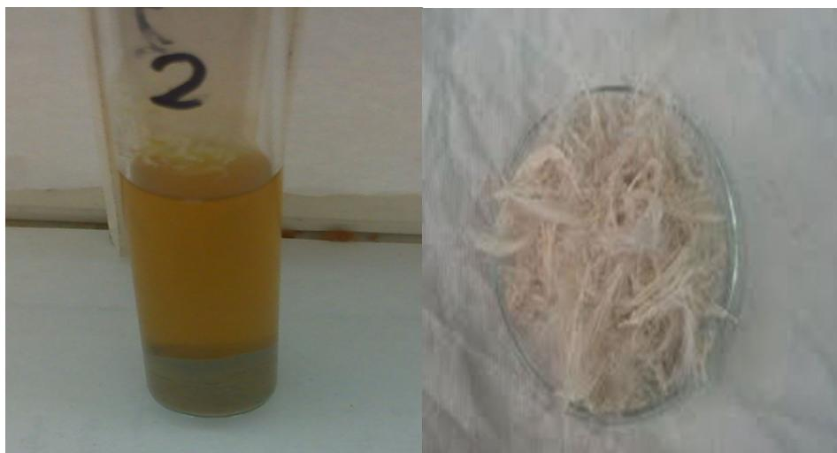
Fig. 2. Untreated (raw) feather (right); and feather hydrolyzed for 200 min (left)
