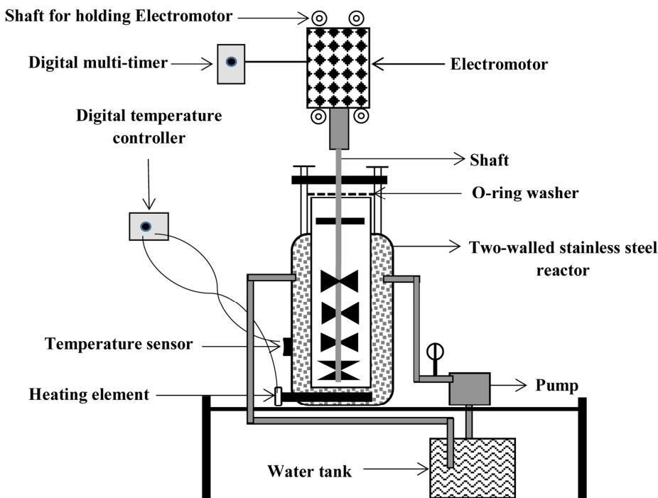
Fig. 1. Schematic of two-walled reactor for hydrolysis of feather
