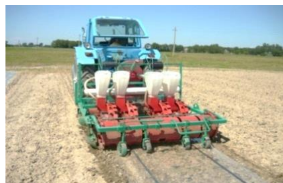
Fig. 8. Combined seeding unit in operation.
