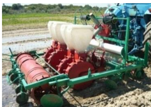
Fig. 8. Combined seeding unit in operation.
