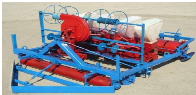
Fig. 6. Experimental prototype of the combined seeding unit.
