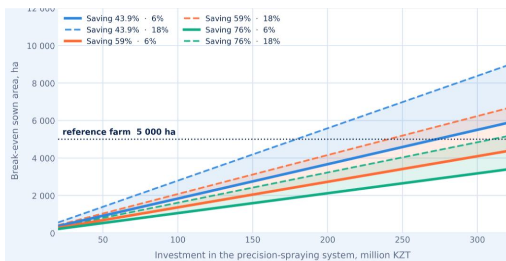
Fig. 5. Minimum farm size at which targeted spraying is economically justified.
