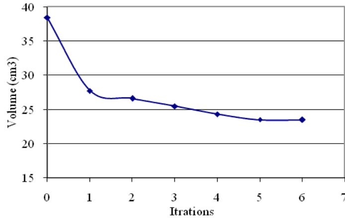
Figure 6. Volume reduction history of the beam.
