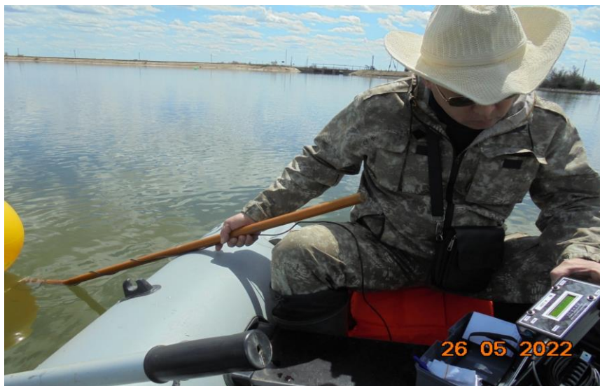
Fig. 1. Measurements of the current velocity by the HMCM-1 device.
