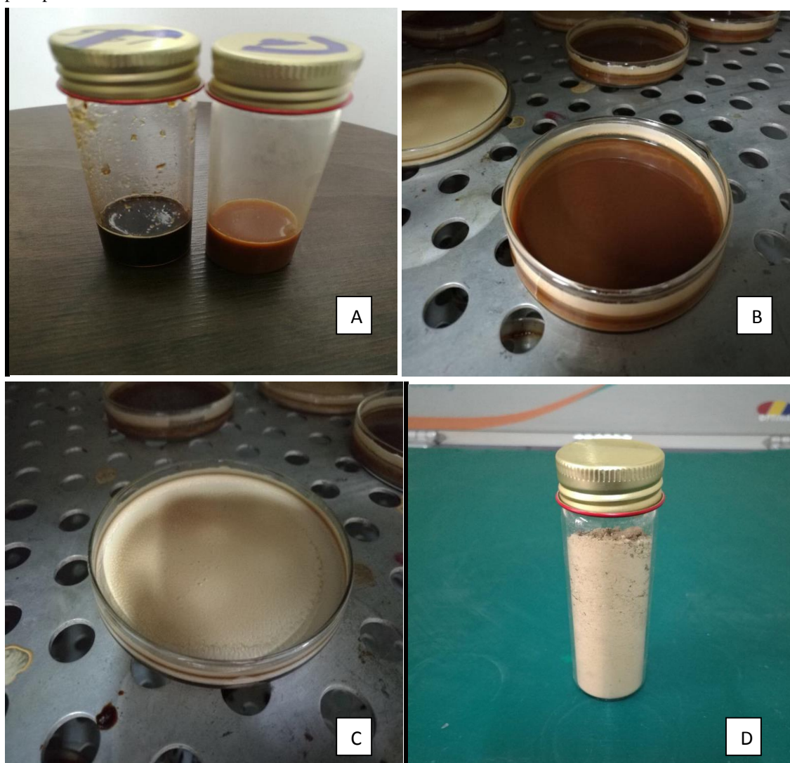
Fig. 2. Step of alcoholic extraction of the plant rhizome; a & b: Both the methanolic and aqueous extracts after filtration; c & d: the dried extract after evaporation.
