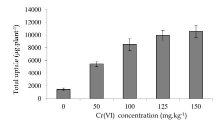
**Fig. 3.** Measured total Cr (VI) uptake (μg plant<sup>-1</sup>) by poplars exposed to different Cr (VI) contents. The exposure period was 7 months. The values are the mean of five replicates for samples. Vertical bars represent standard deviation.
