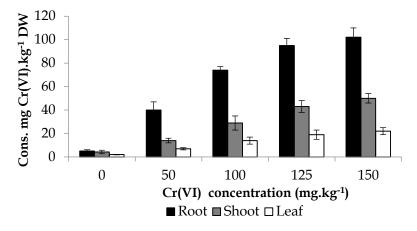
**Fig. 2.** Measured total Cr (VI) concentration (mg kg<sup>-1</sup>) in plant organ of *P. nigra* L. exposed to different Cr (VI). The exposure period was 7 months. The values are the mean of five replicates for samples. Vertical bars represent standard deviation.
