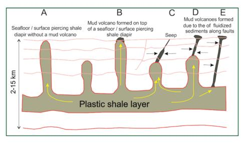
**Fig 8.** Basic mud volcano formation. A) Clay diaper, B) seafloor-piercing clay diapir - a mud volcano. C) Sea floor seepage. D, E) mud volcanoes formed due to rise of fluidized sediments along faults (adopted from Milkov, 2000).
